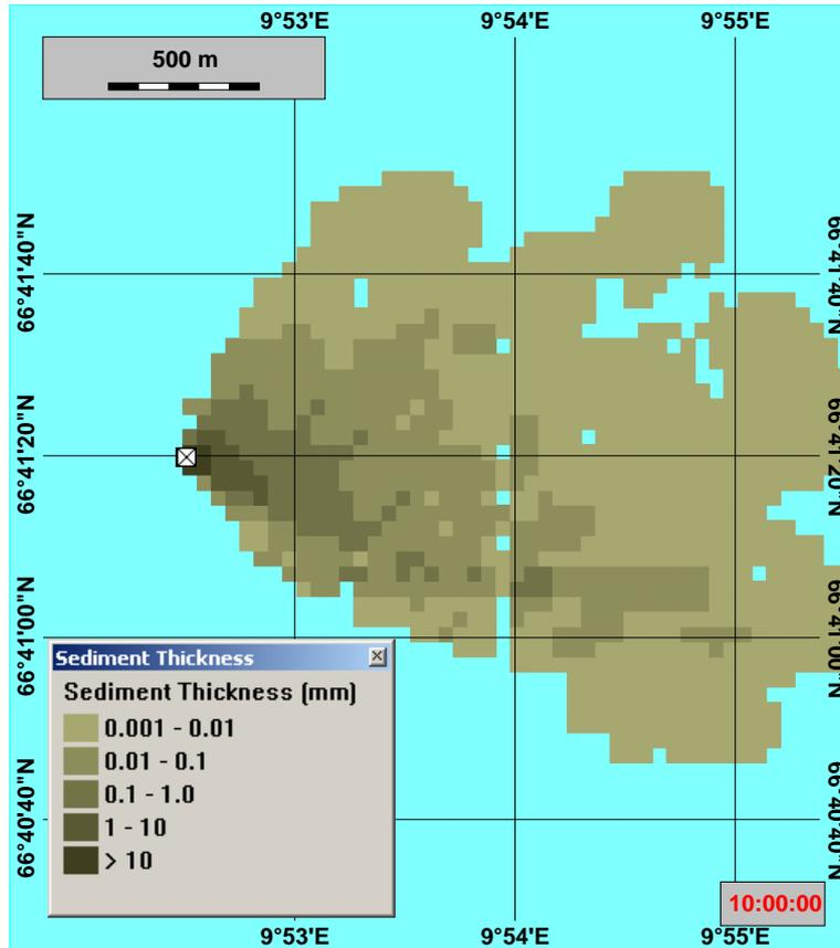
Figure 4.1 Deposition of discharge (layer thickness) at the end of the discharge period (after 10 days).
