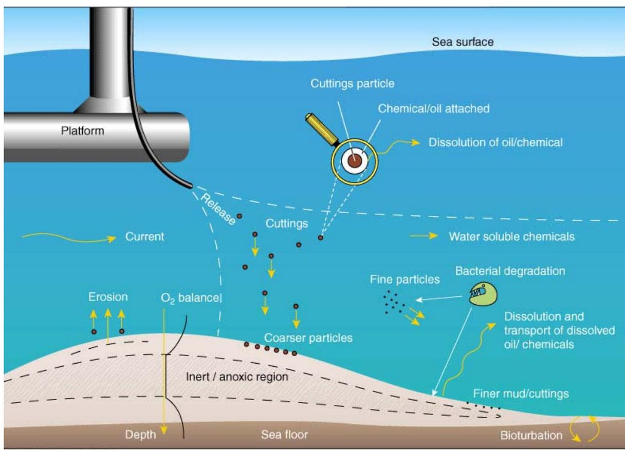
Figure 2.2 Overview of short- and long-term disturbances of drilling discharges
