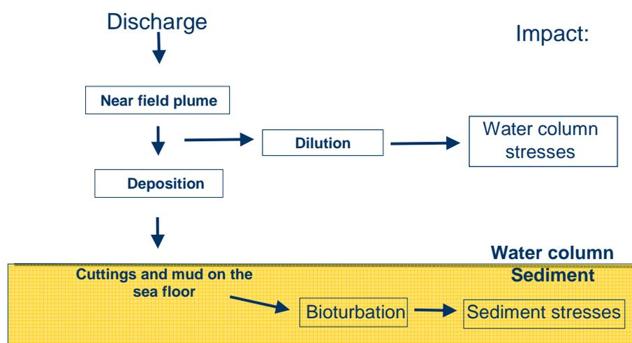
Figure 3.2 Layout of the model structure for calculations of potential impact.
