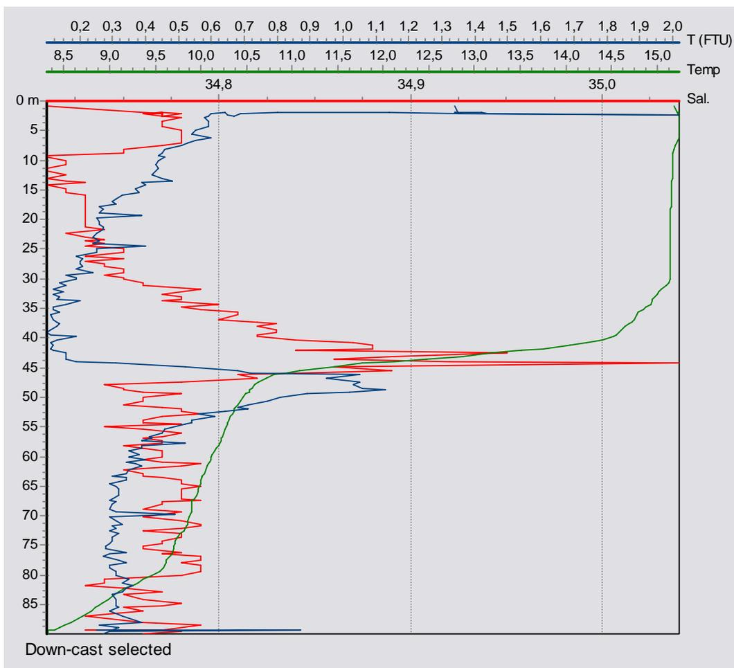
Figure 5.2 CTD profile close to the discharge site 10 September 2003, at time 1200. The vertical profiles collected at shell cage location B are assumed to be representative for shell cage location A as well. Turbidity (blue), temperature (green) and salinity (red).
