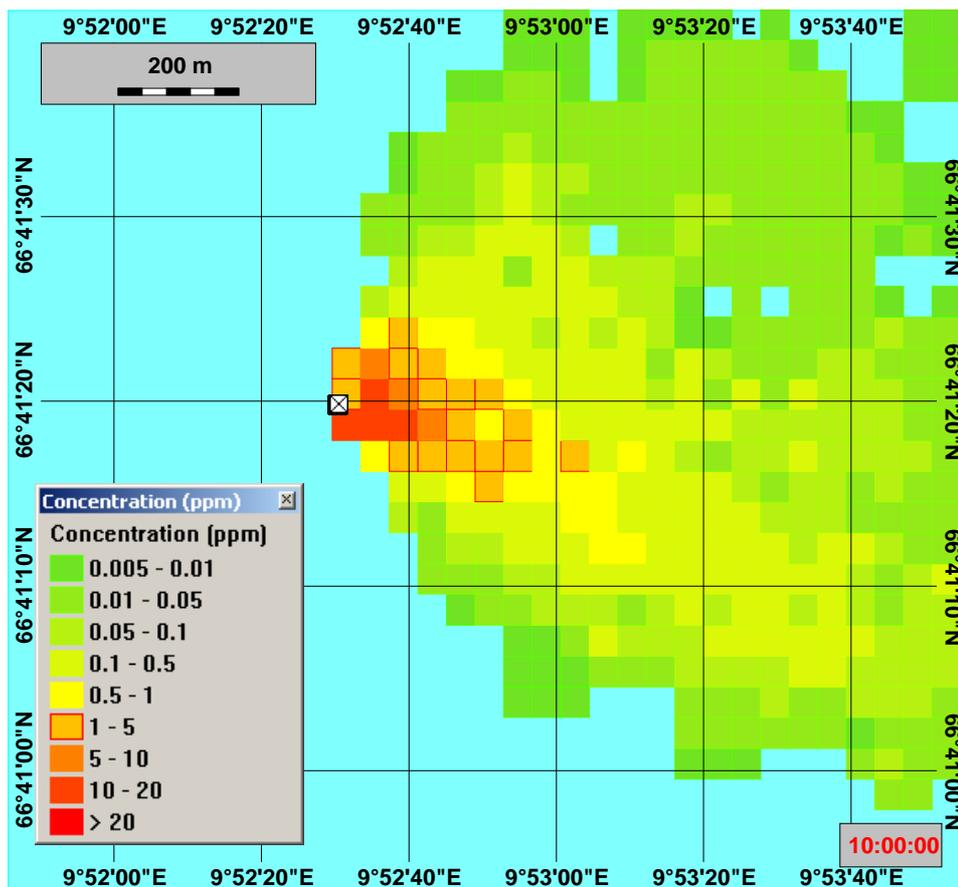
Figure 4.3 Concentration of the “dope” chemicals in the sediment layer at the end of the discharge period (10 days). Max concentration of the “dope” is about 16 ppm (mg/kg sediment)
