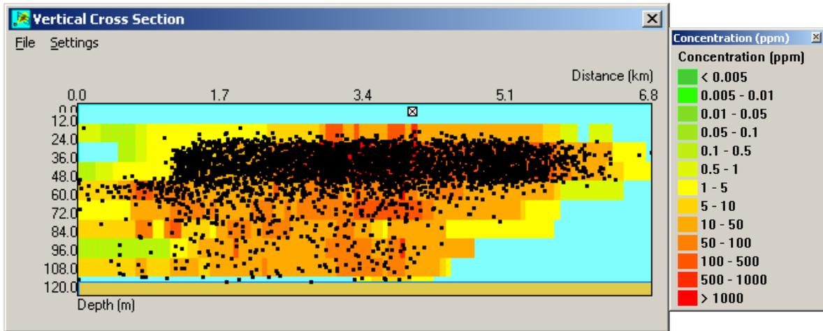
Figure 5.1 Numerical modeling with the revised DREAM model. A vertical cross section of the plume calculated for the SVAN field release. The discharge point is shown with a cross inside a square (with a cross inside) at 5 m depth at the figure. The near field plume from the discharge will sink down to about 35 – 40 m depth. At this level, the discharge spreads out and is transported away with the currents.
