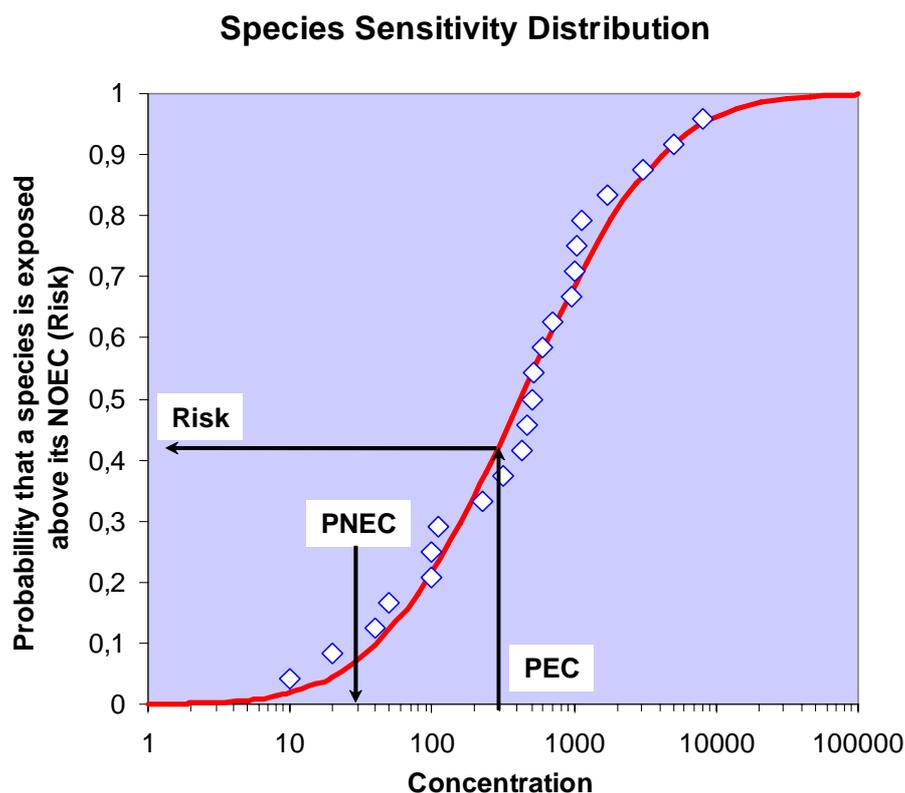
*Figure 3.3 An example SSD; The PNEC corresponds to a probability value (PAF) of 5%. At any PEC a Potentially Affected fraction of Species (PAF) can be calculated.*
