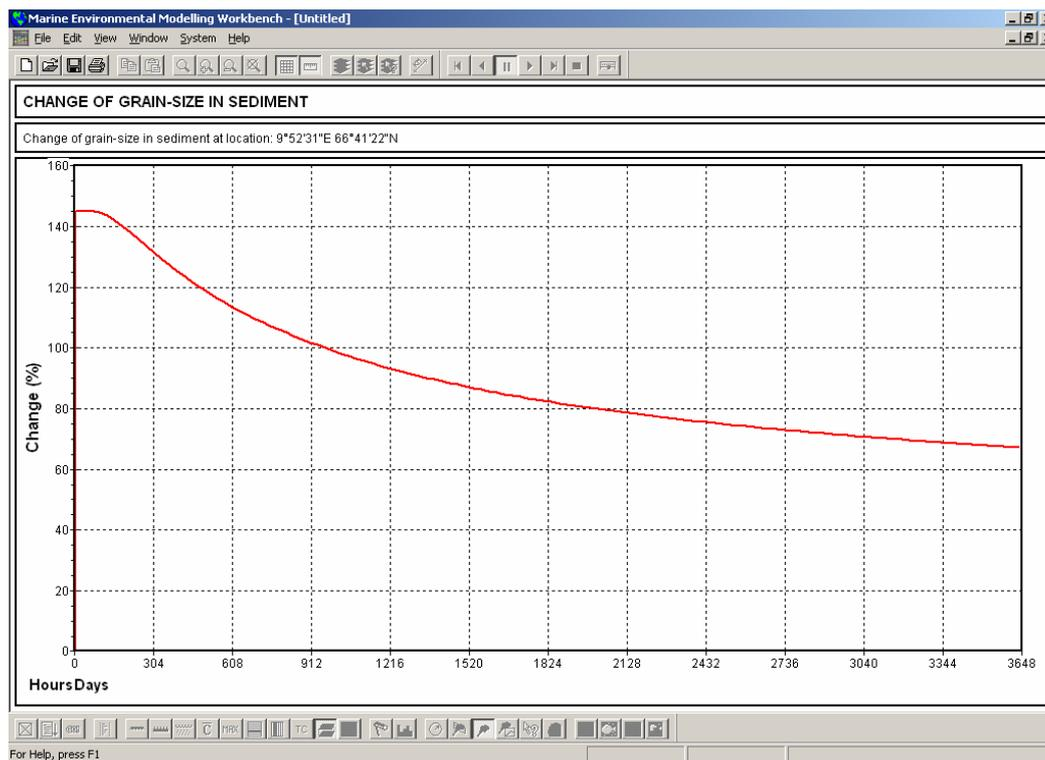
Figure 4.8 Time series for change of grain size for one selected grid point. The reduction of grain size change with time is due to effects from bioturbation, mixing the added particles downwards while the original particles mix towards the sediment surface.
