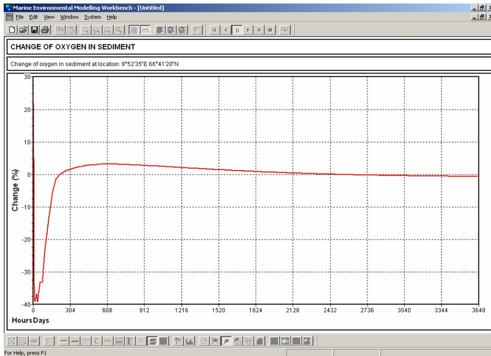
Figure 4.6 Oxygen depletion calculated as a function of time for the grid point with the largest concentration of the lubrication chemicals. Horizontal scale in days. The PNEC level of 20 % reduction of the oxygen content in the sediment layer is surpassed for a short time period (some months) in the beginning of the sediment impact simulation period.
