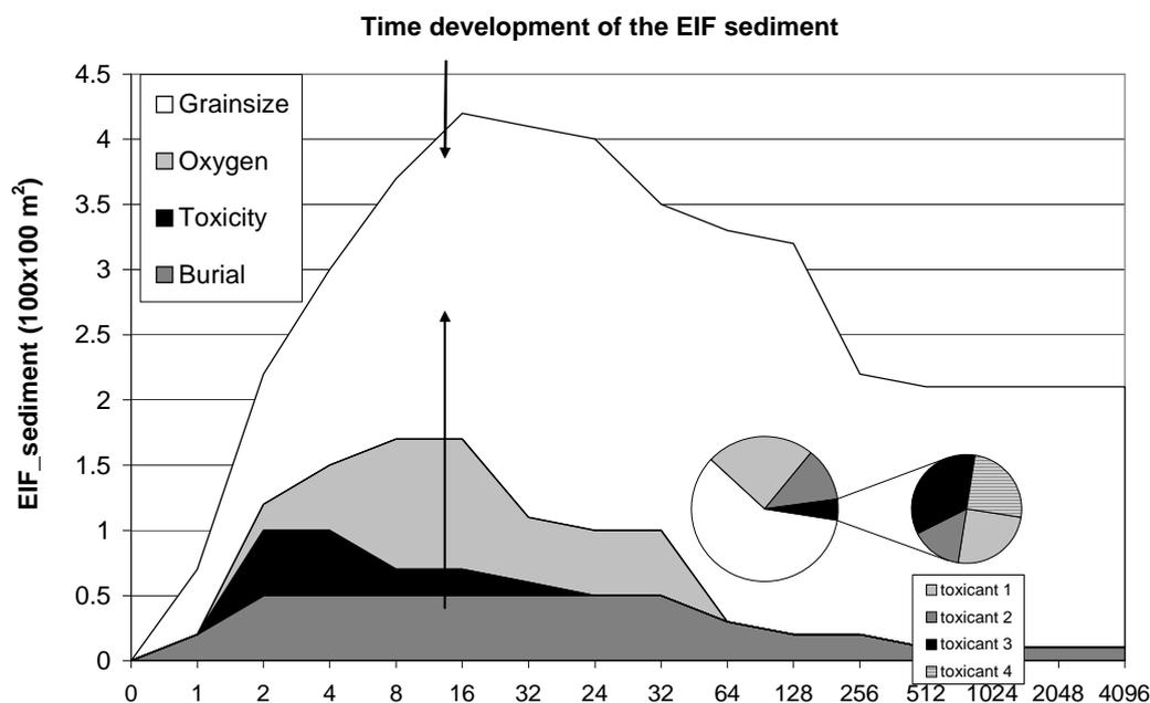
Figure 3.6 Graphical presentation of an example of the influenced sediment area (represented by  $msPAF > 5\%$ ) and the contribution of each stressor to the overall risk related to this theoretical drilling discharge.
