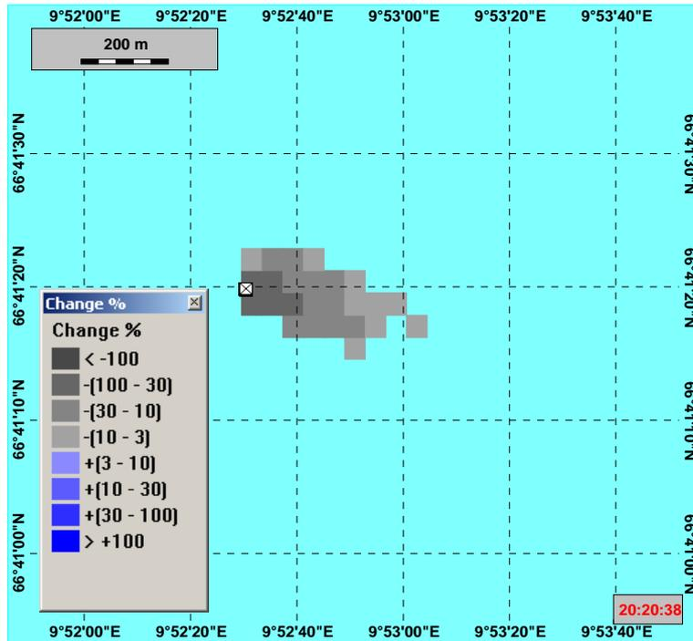
Figure 4.5 Oxygen depletion in the sediment layer after about 20 days of simulation time, caused by the degradation of the lubrication chemicals.
