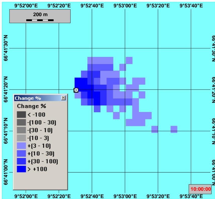
Figure 4.7 Change of grain size in the sediment at the end of the discharge period. The median grain size is averaged over the upper 3 cm of the sediment layer.
