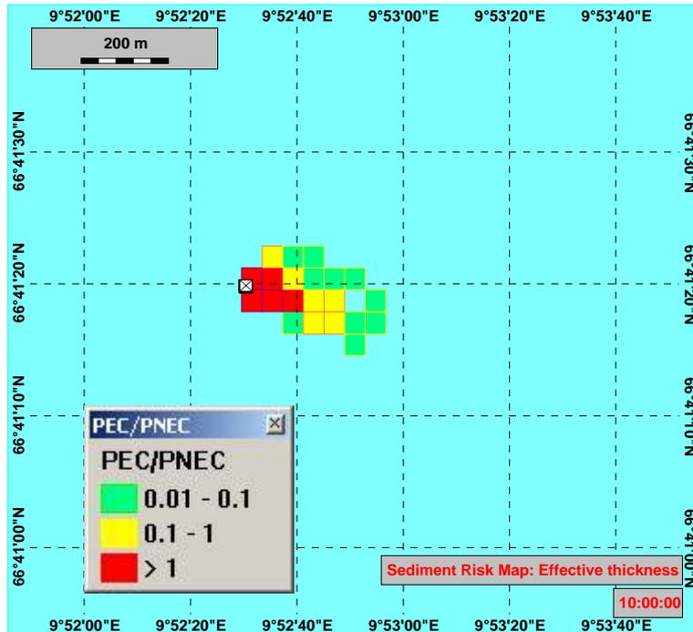
Figure 4.2 Grids that exceed the PNEC level for burial at the end of the discharge period (red color). Grid points are approx. 50 x 50 m.
