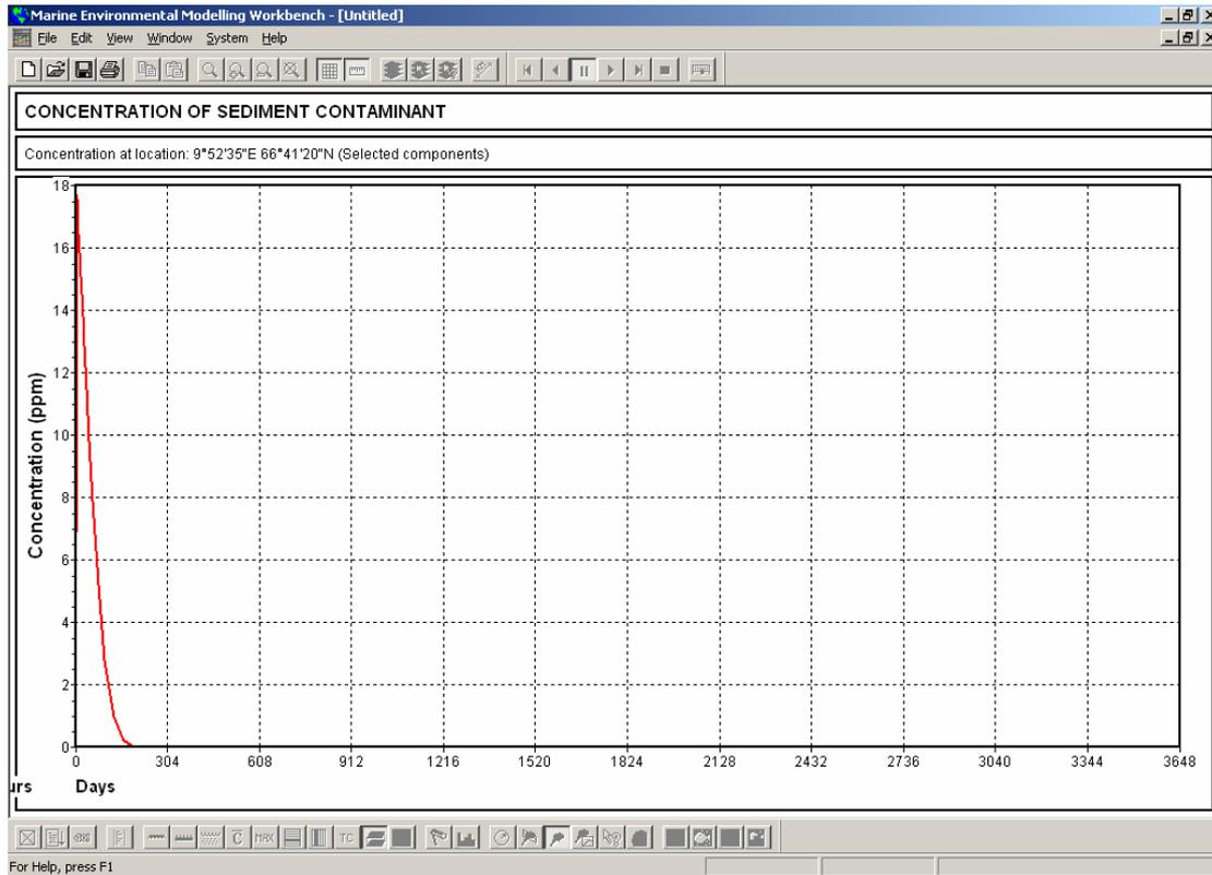
Figure 4.4 The time development of the “dope” concentration in the sediment layer for the grid with maximum concentration. Horizontal time scale in days. The concentration is biodegraded down to zero within about 6 - 8 months.
